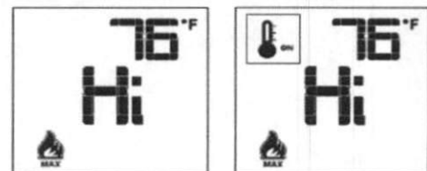
Figure 11.7c, Deactivated / Activated Thermostat
